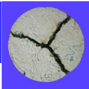
c -Failure cone with splitting cracks Bolt did not pullout d_b=10\text{mm} , v_f=0.8\% , l_f=16\text{mm}
