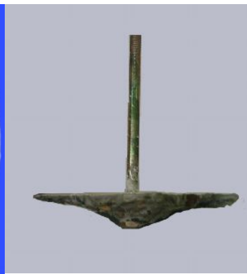
a -Concrete Failure cone d_b=8\text{mm} , v_f=0\% , h_{ef}=25\text{mm}
