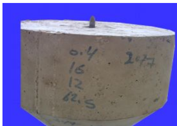
d- Steel Failure , d_b=12\text{mm} v_f=0.4\% , l_f=16\text{mm}
